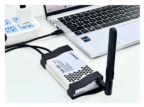
Figure 4 schematic diagram for a typical setup of SAE-200.
